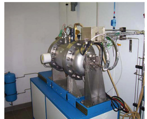
Fig. 4. Schematic of the high temperature–high pressure corrosion test equipment (a), and view of the furnace (b).
